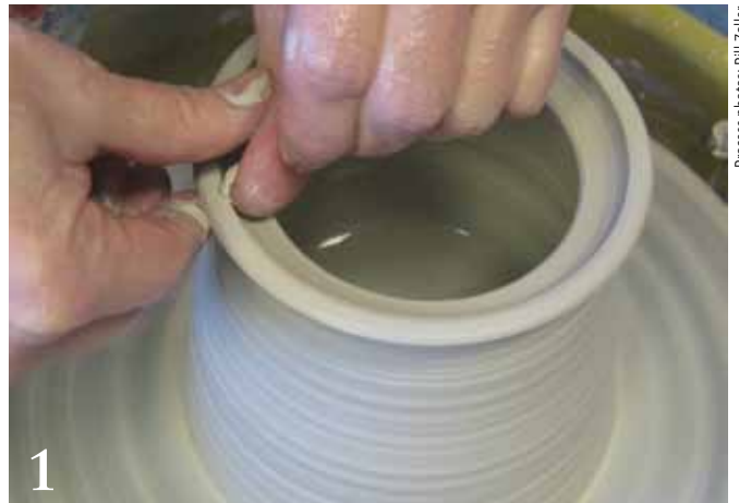
1 Throw a cylinder for the body of the teapot, leaving a thickened rim. Split the rim in half to create the gallery.
