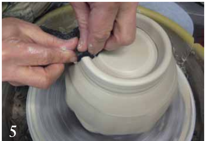
5 Add an extra coil onto the bottom and throw it into a tall foot. The diameter of the foot should echo the rim.
