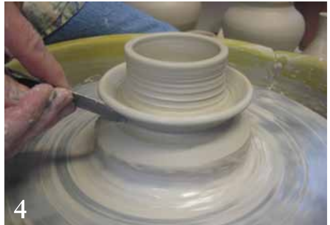
4 When forming the lid, split the rim from the flange, then remove extra clay from underneath, making a curve.
